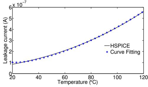
**Figure 1: Comparison of leakage of a TSMC 65 nm process MOSFET from HSPICE simulation with its curve fitting result using (2).**
