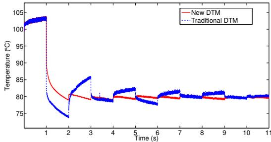
**Figure 4: The transient temperatures of C32 using the new DTM (with 5 expansion points) and traditional DTM. Both methods have  $N_p = 2$  and  $N_c = 1$ . The temperature target is set as 80 °C. Both DTM methods are activated at 1 s.**
