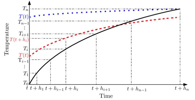
**Figure 2: The sketch map of the PWL method for one control step.**  $T_1, T_2, \dots, T_n$  are the potential Taylor expansion points.  $t, t+h_1, \dots, t+h_n$  are the potential local linear model switching time points. The black solid line is the extreme temperature trajectory. The red dashed line is a common temperature trajectory. The blue dot line represents the temperature trajectory which is already very close to the target at time  $t$ .
